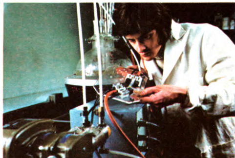
Photocell monitoring to control chemical process of organic resin phosphor synthesis.
