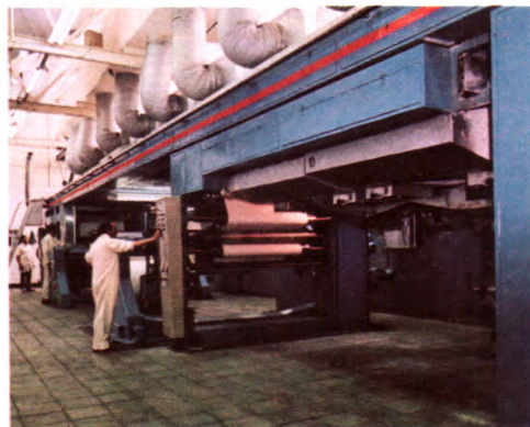
Modern high quality coating and gumming machine. Used for phosphor and other coatings.
