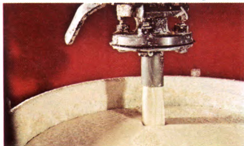
Filtration of phosphor coating mix through very fine mesh.
