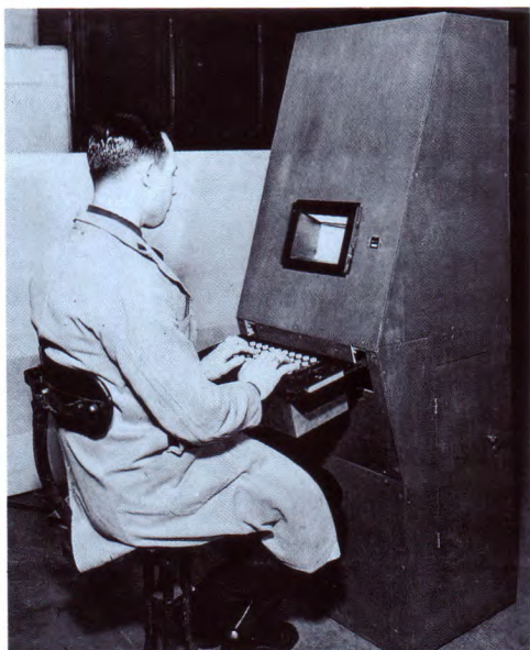
1948. Dummy desk for trials with different keyboards to be used on the 'Interim' machine.
