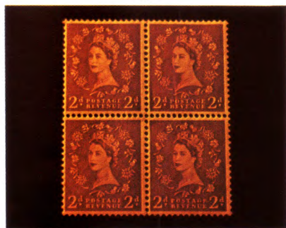
Fig 8: Stamps printed on hand made paper impregnated with yellow-emitting phosphor
