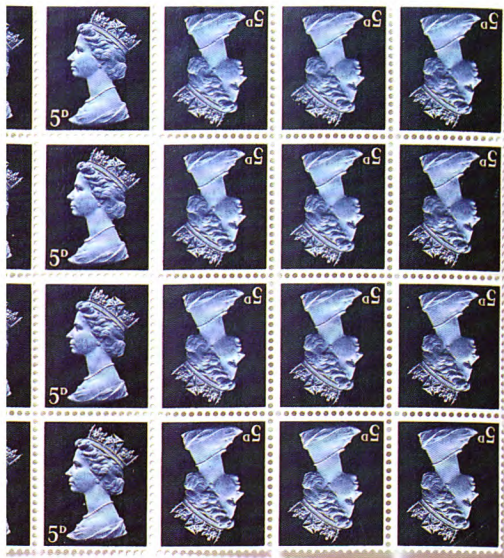
Far left, a 'dry print' error arises when the press is inked-up or at the end of a run, when ink is running out. Left, an example of a paper fold. Above, this block from a booklet sheet shows the layout of sheets from which booklets are guillotined.
