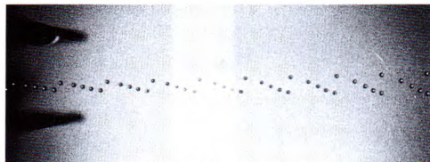
4. Jet printers have enabled mail to be postcoded at processing speeds of up to 5 metres per second. In the continuous ink jet printing process a stream of droplets is guided towards the paper surface by an electrostatic field.
