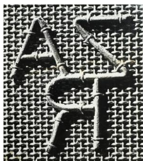
Wired watermark mold used to produce paper.
