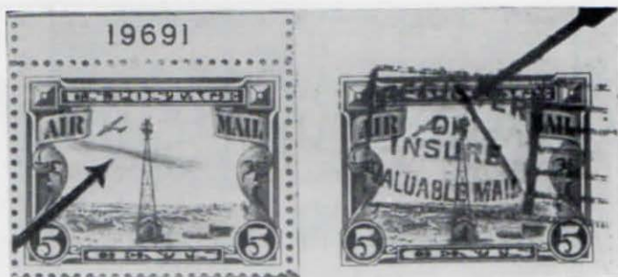
Fig. 21. (Left) A plate scratch that caused the appearance of a red streak across the sky. (Right) A diagonal plate scratch produced a blue streak.
