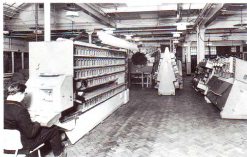
SPLSM on trial at Southampton in 1957, with prototype segregator and the first ALF.
