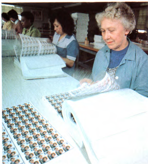
The final checking department where any minute errors in colour registration and perforations are spotted.
