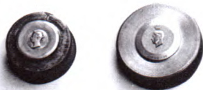
Edmund Dulac's head of King George VI developed at the Mint as an embossing die punch matrix
