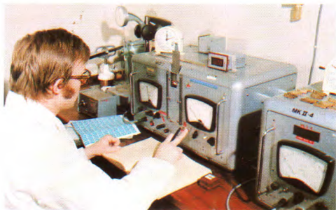
1 Routine measurement of phosphor brightness
