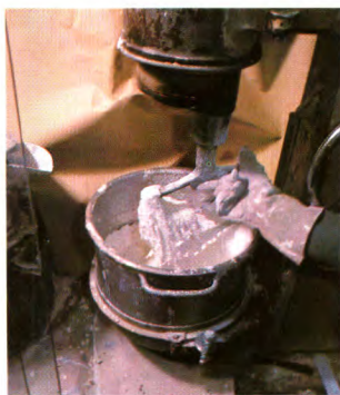
6 First stage of manufacture of TAP stamp phosphor at Harrisons. The chemical reaction
