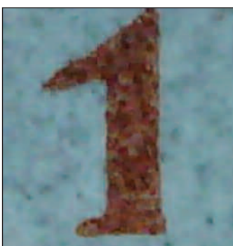
Figure 24 Complete break of the bottom right foot serif of the left numeral “1.”
