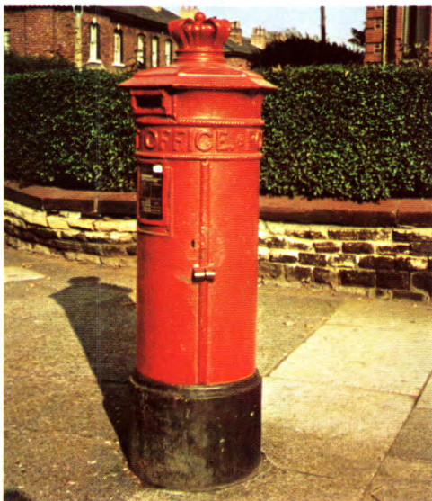
No. 7: This old Victorian pillar box with the crown on top is known as a 'Liverpool Special' because it was designed and manufactured especially for use in Liverpool to cope with the heavy postings experienced in that City. Made by Cochrane & Company of Dudley, the boxes were introduced in 1863 and two of them are still in use today.
